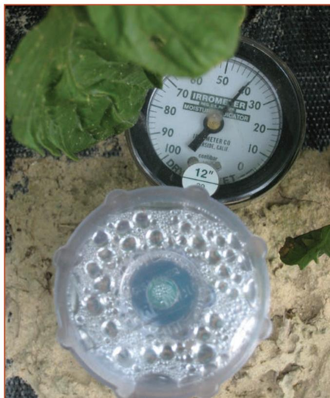
**Figure 13.** A tensiometer can be used to monitor soil moisture.
